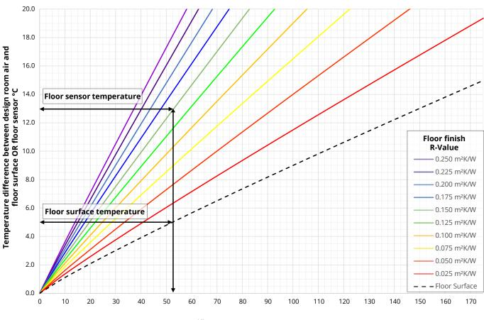
Floor sensor setting for target heat output
