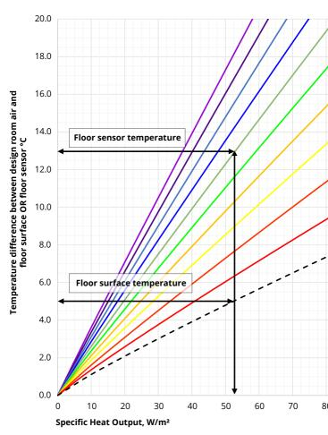
Using the graph above it is possible to get the specific heat output of an eUFH system based on the temperature difference between the design room air temperature and the floor surface or floor sensor temperature by floor finish.
