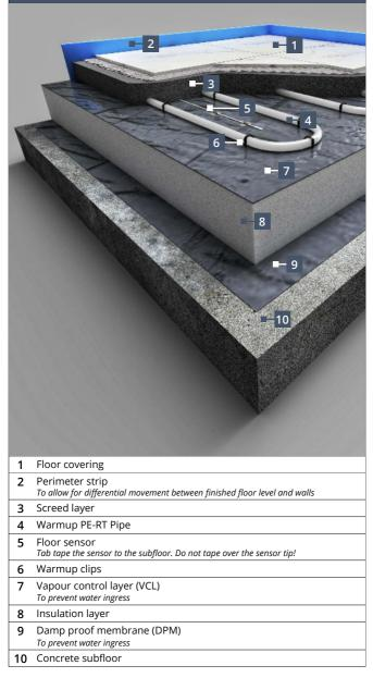
The concrete subfloor must be clean, level, solid, structurally sound and dimensionally stable. Ensure the subfloor is prepared to an SR2 standard (SR2 - the maximum permissible departure over a 2 m straight is 5 mm).
