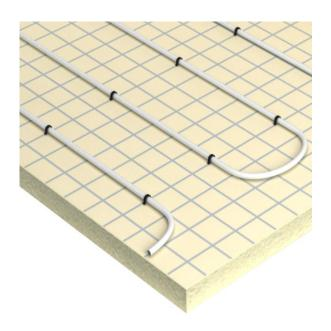
The Warmup Clypso PIR Insulation is a rigid polyisocyanurate foam core board with aluminium foil composite on both sides. The insulation boards are provided in 2400 x 1200mm sheets and come in 25,40,50,60 and 75mm thicknesses.
