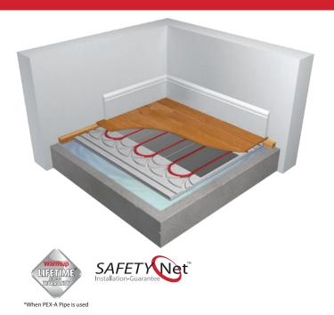
Warmup Total-16 is a lightweight, heavy duty insulation system comprised of three components: straight, multi-feed and return boards. These boards are made of high density EPS, able to withstand 40 Tonnes/m². The straight boards come with aluminium heat diffusion plates as an integral part of the board. Total-16 significantly speeds up installation time for both, new-build and refurbishment projects, where floor zone height is at a premium.
