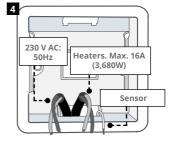
Install a 50 mm deep electrical back box in your preferred thermostat location. Pull wires (heater, supply and sensor(s) through back box and complete terminal wiring.
