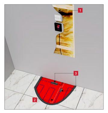
The supply to the thermostat MUST be protected by a 30mA RCD or RCBO at all times. Time delay RCD's or RCBO's must not be used. No more than 7.5 kW of heating should be connected to each 30 milliamp RCD or RCBO. For larger loads, use multiple RCD's or RCBO's.
