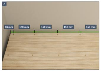
Screw the plywood covering into the Econna-12 panels using 25 mm wood screws, 18 mm in from the edge of each plywood sheet and then at 150 x 150 mm centres, ideally in the centre line between the pipe runs.
