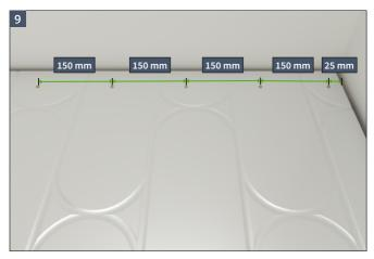
Screw the Econna-12 panels to the joists using 55 mm wood screws,
