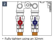
• Ensure pipe is fully inserted into fitting. Hand tighten.
