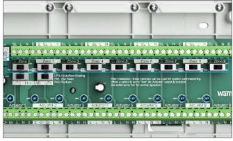
Warmup actuators are supplied latched open for easy mounting on the manifold. They need to powered on for at least 2 minutes to fully open them and disengage their latches so that they can close the valves.
