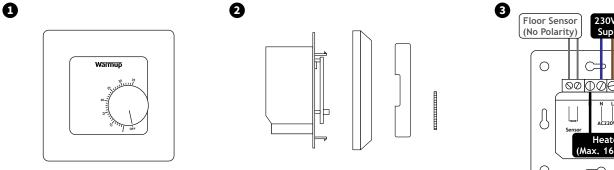
Gently remove the dial using a small screwdriver, followed by the cover inserting a small screwdriver into the release clip Remove the front fascia by unclipping from the base and placing somewhere safe
