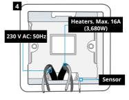
Install a 50 mm deep electrical back box in your preferred thermostat location. Pull wires (heater, supply and sensor(s) through back box and complete terminal wiring.
