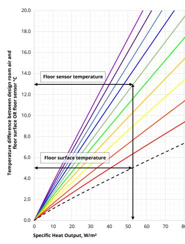
The room with the highest water temperature requirement sets the design water temperature for the whole system based on the calculations from the previous section.
