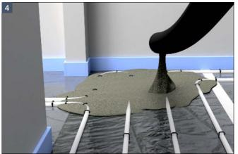
Apply the screed layer referring to the screed manufacturers instructions for mixing, drying and curing information.
