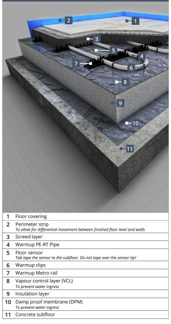
The concrete subfloor must be clean, level, solid, structurally sound and dimensionally stable. Ensure the subfloor is prepared to an SR2 standard (SR2 - the maximum permissible departure over a 2 m straight is 5 mm).
